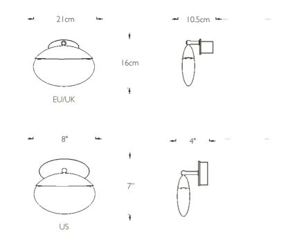
wall light: oval back plate -  $10 \text{cm w} \times 4.3 \text{cm d} (6.5'' \text{w} \times 1\frac{1}{4}'' \text{d to fit } 2'' \times 4'' \text{J-box})$
